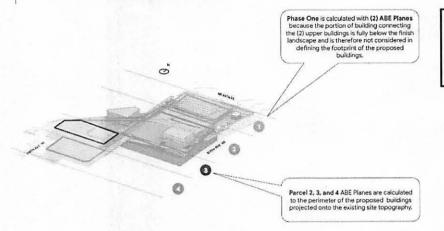
The plan extents of the "Average Building Elevation" for zoning shall be traced around the perimeter of portions of buildings with walls 4' or tailer above finished grade. These footprints are projected onto the existing site topography to determine the ABE for each building. The Northern Mid-Block Connection is at grade, so there will be two ABE calculations for the Phase 1 structure.
